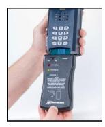
Slide the **Power** switch on the power paddle to the **ON** position. The green **POWER** light will illuminate.
